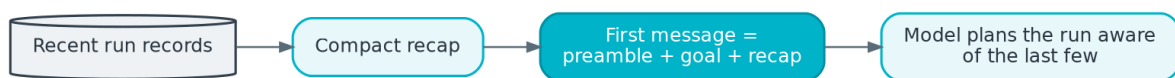
Figure 8. Cross-run memory. Each run is seeded with a recap of the last few.
